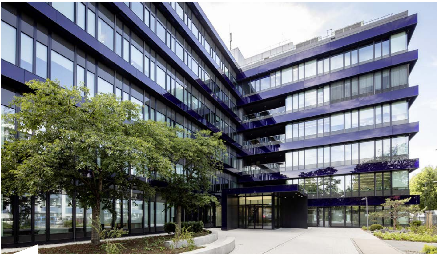
The Building "BAU 11" in Munich was given a modern, visually striking façade with blue glass façade bands and Infrastop solar control insulating glass.
