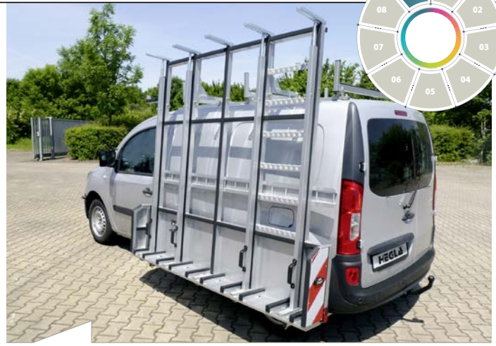
A van with removable Hegla external reeving and luggage racks offers plenty of space for cargo and is, due to its compactness, suitable for city traffic.
