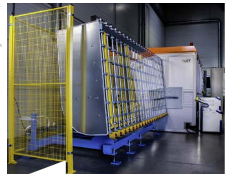
With the new 4Jet lasers, flexible, laser-based filamentation and separation of glass is possible.
