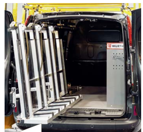
The pull-out interior reeving allows IG units and windows to be loaded in a way that causes less strain for the workmen. Still, they are well protected inside.
