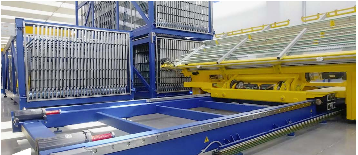
Forvet's Sortiflex two-tier compartment storage system doubles the number of storage spaces available in the same footprint, increasing storage volume without taking up more valuable production space.
