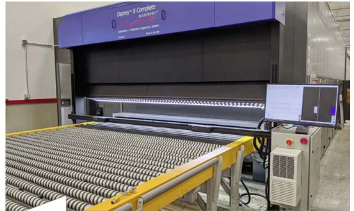
These days, glass processors demand that the scanners used should detect distortions in the glass as well as any anisotropies.
