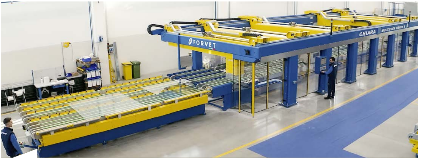
The Chiara Multiflex Heavy is a flexible and space-saving solution for edge processing. Straight edges and borders – even with non-rectangular contours – in the brilliant quality of cup wheel technology.
