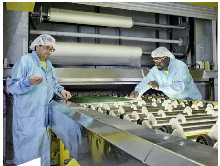
Production of fire-resistant glass in the clean room at Vetrotech Saint-Gobain in Würselen.
