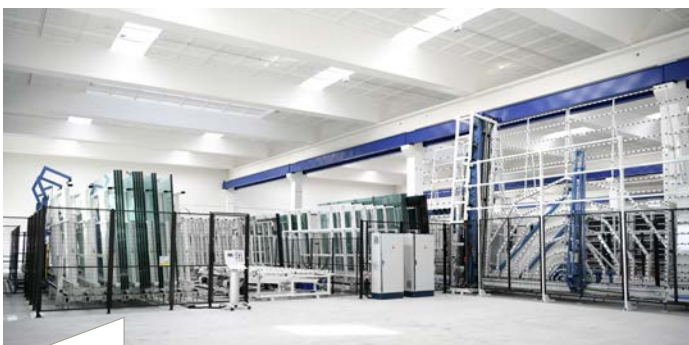
The new production is highly automated: The basic glass, including laminated safety glass, are sent from an automatic warehouse (I) on to the vertical cutting line.
