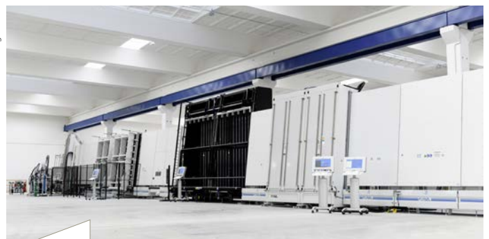
With the High-Tech IG line, high-quality window and facade glass can be produced in formats of up to 6,000 × 3,300 mm, even 4-fold structures are possible.
