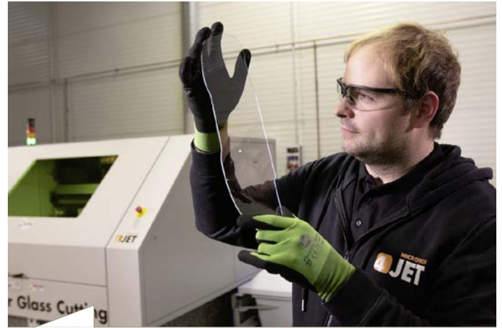
The laser can also take over parts of the glass processing while it is cutting. Here, a filamented and separated display glass from a Pearl laser cutting system.
