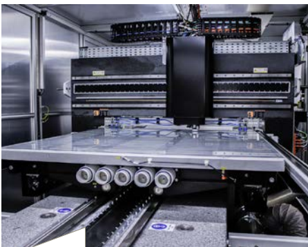
Inside view of a Pearl L laser from 4Jet with substrate table and processing head.
